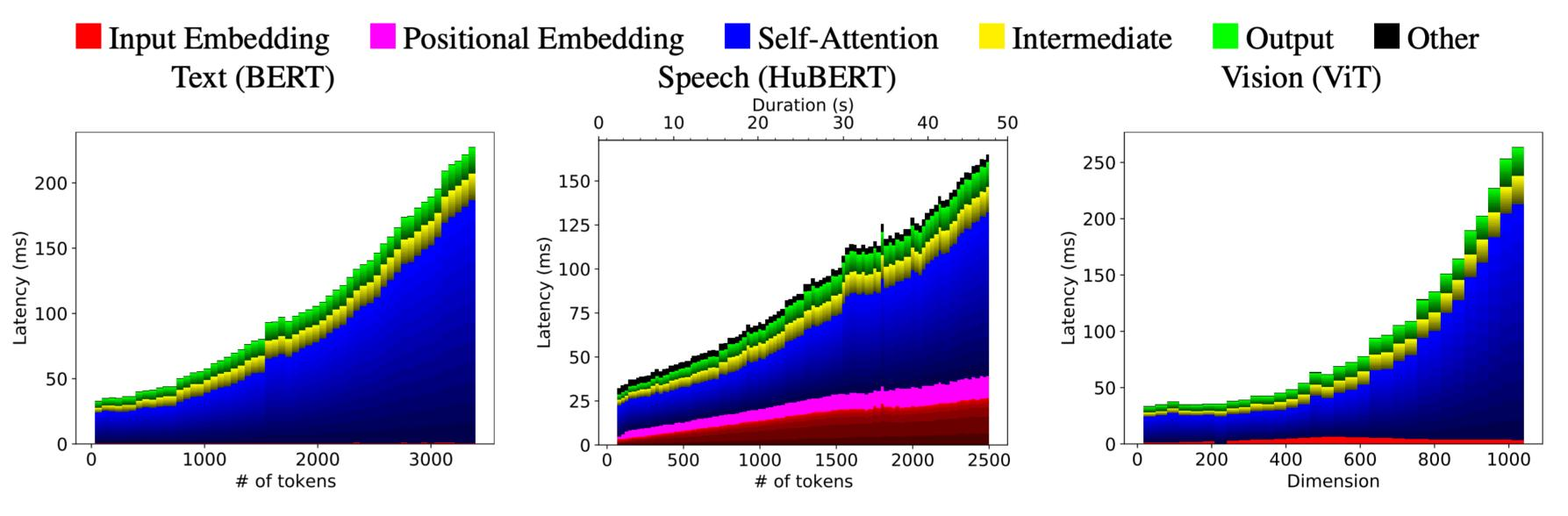
Figure 1: Layerwise latency of different vanilla Transformer architectures in inference mode.
